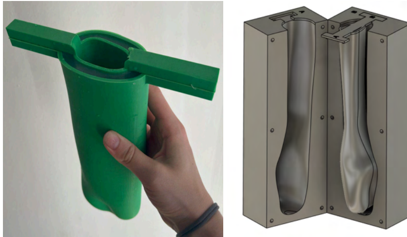
Figures 45 and 46 Initial Silicone Mold Design, Final Silicone Mold Design
